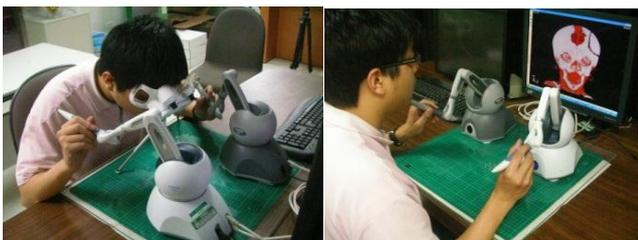
Figure 21. Two-arm manipulation and head-mounted display.
