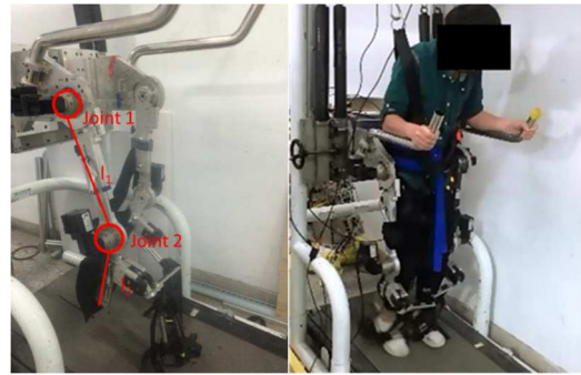
Fig. 1. 2 DOF Manipulator based Exoskeleton in the real view.
